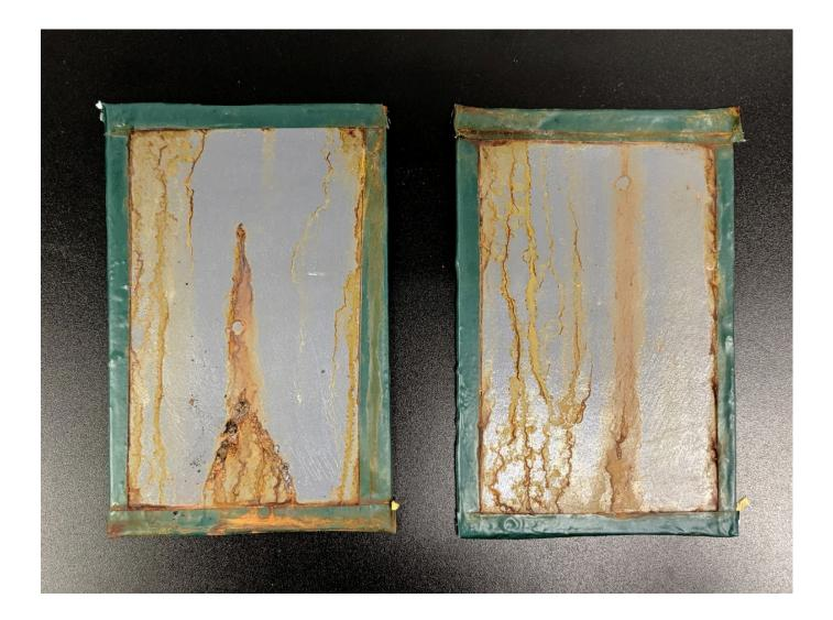
CRS - Color Variant (GRAY) 1500 Hours ASTM B117 Salt Spray
